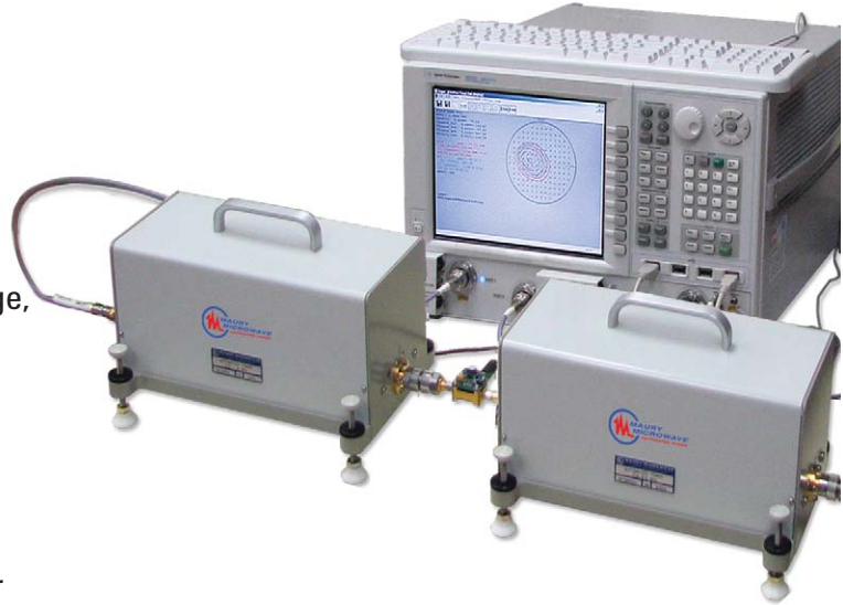
PNA-X network analyzer with Maury load-pull tuners
